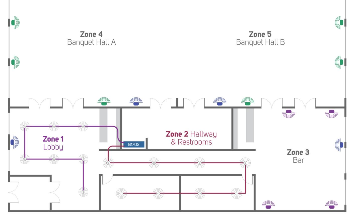
Large Application – 5 Zones **BSP200** Indoor Speakers x 4 BSW150 Network Subwoofers x 3 **BSP1000** Indoor/Outdoor Speakers x 8 **B170S** Network Streaming Amplifier - 70/100 V Mode © Ceiling Speakers with 70/100 V transformer **CP100** Wall-mount Control Panel (optional)
